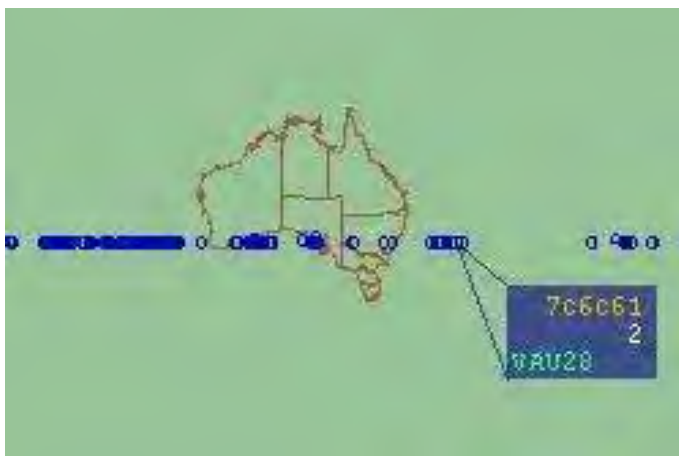
Figure 1 - Track Jumping problem with TPR901
