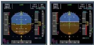
Figure 1 PFD in CONF3 and PFD in CONF3 after retraction of the flaps. The PFD shows the aircraft in LAND mode and the Autopilot (AP) is engaged.
