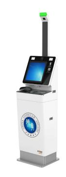
a self-service, all-in-one kiosk for collection of biometric information, usi PKD and optical anti-counterfeiting technology
