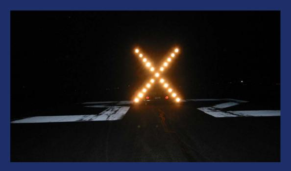
Lighted X's are very effective during low visibility conditions and at night when the runway lights must be illuminated for maintenance or during snow removal operations.
