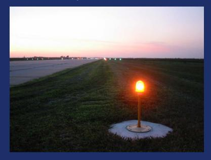
When the runway threshold is temporarily moved for construction and the runway is open at night, the caution zone lights marking the last 600 m (2000') of runway will need to be adjusted. If runway center line lights are present, they will need to be placed out of service.
