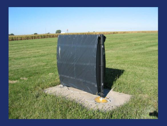
When the runway threshold is temporarily moved for construction, the runway distance remaining signs in the opposite direction must be covered as they no longer provide accurate information
