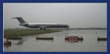
When inspecting construction areas, Inspectors should check for adequate unserviceability markers, warning signs and potentially misleading or confusing pilot visual aids
