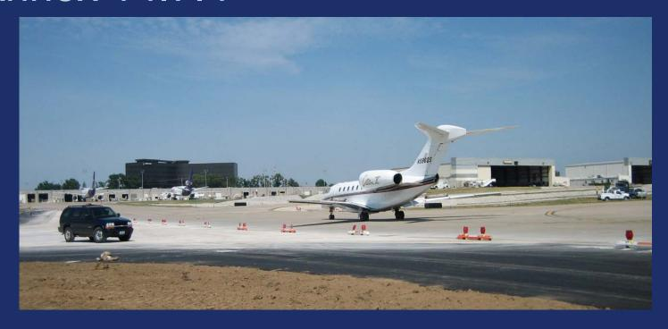
Unserviceablity markers shall be displayed wherever any portion of a taxiway, apron or holding bay is unfit for the movement of aircraft but it is still possible for aircraft to bypass the area safely. On a movement area used at night, unserviceability lights shall be used.
