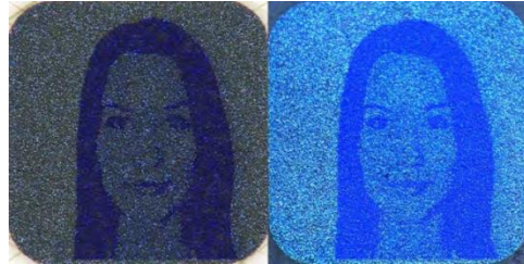
Figure 0–7: Passport (LVA, P, 1, 2015): “Negative” personalization through laser engraving under different viewing angles in visible light
