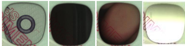
Figure 0–10: Passport (SWE, P, 1, 2012): Window feature with variable content; from left to right: inner front cover; reader housing; fingertip; glare induced by incident light
