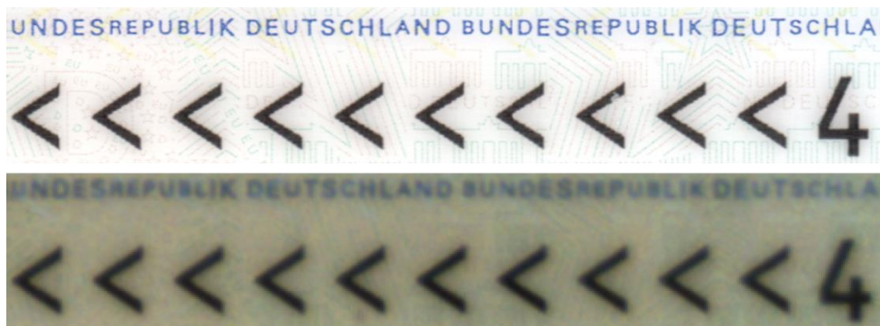
Figure 0–9: Passport (D, P, 1, 2017): Comparison between a high-resolution image of the microtext (1000 ppi) and an image of the same microtext taken from a full page reader (nominal 400 ppi)
