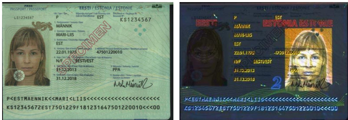
Figure 0–12: Passport (EST, P, 1, 2013): Verify the facial image in the visible light image against the one printed with UV-luminescent ink
