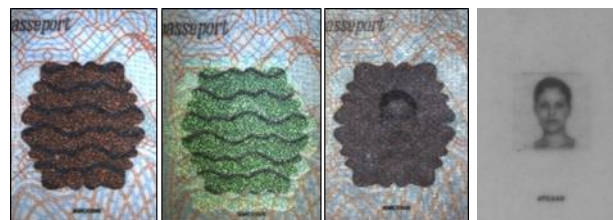
Figure 0-6: Passport (HUN, P, 1, 2006): Personalized OVI viewed under two different angles, under transmitted light and under IR light
