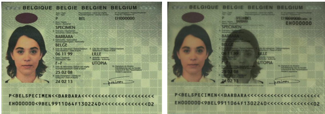
Figure 0–11: Passport (BEL, P, 1, 2008); left: plain data page; right: data page with an overlay of the transparent sheet for visual inspection
