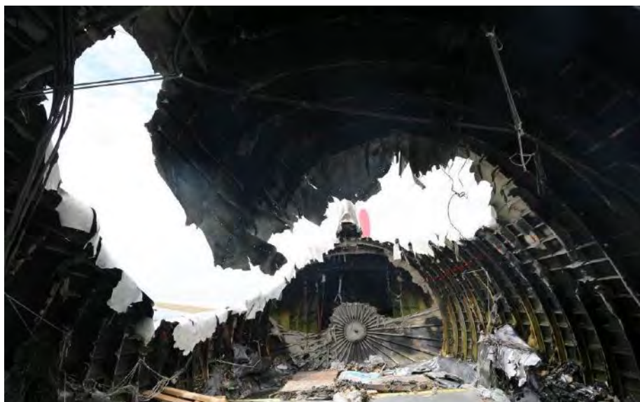
Figure 63 The Aft Pressure Bulkhead and Aft Main Deck Compartment Damage
