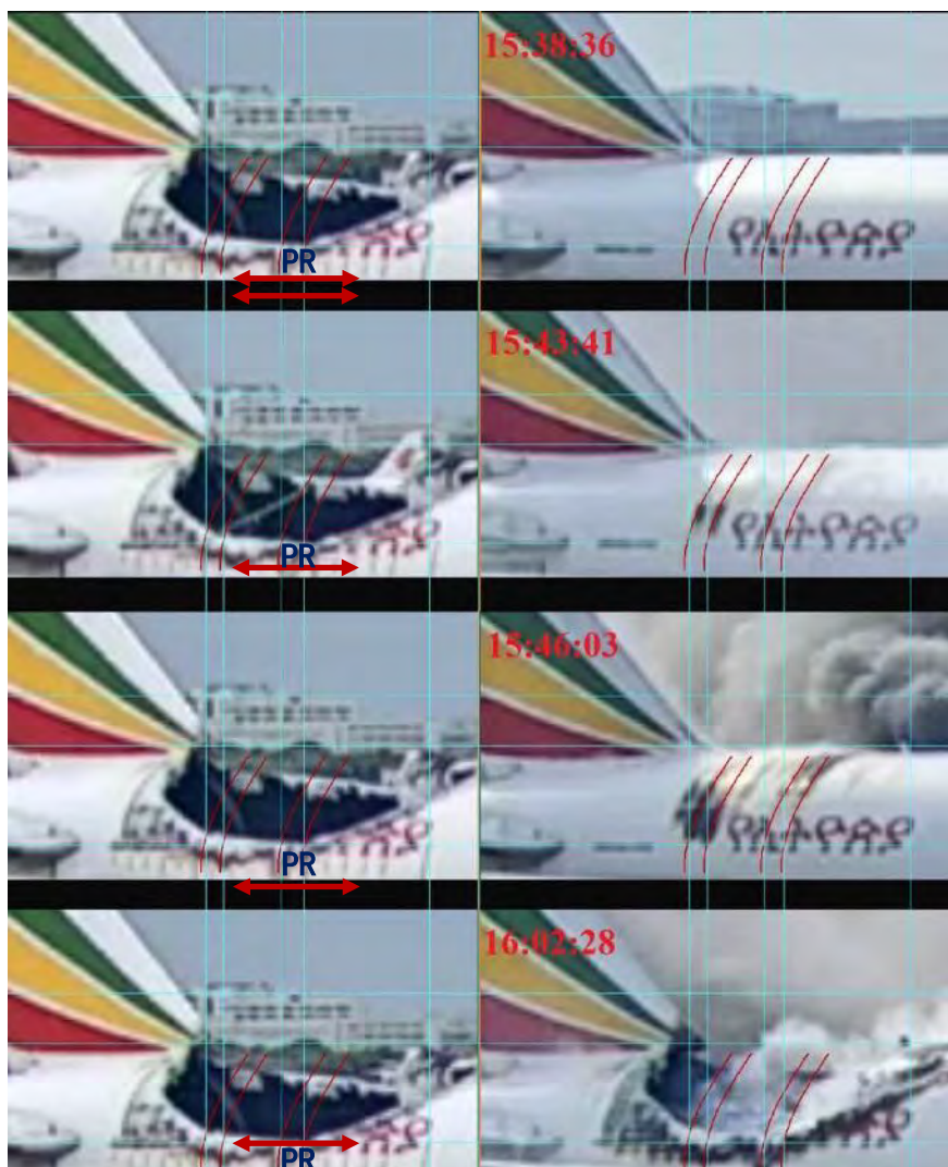
Figure 69 Comparison between the CCTV Footage of Parking Position No.307 (right) and the Post fire Aircraft (left)
