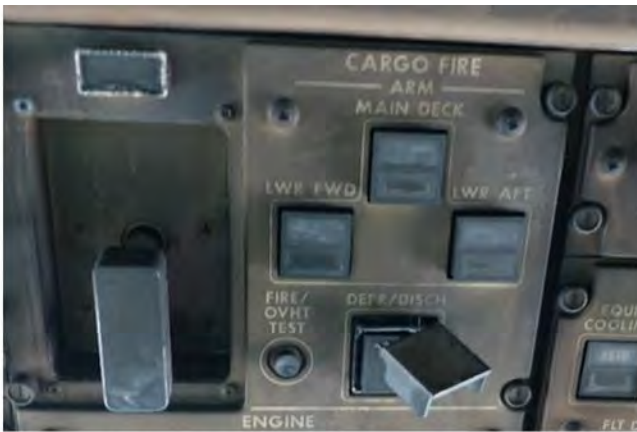
Figure 18 Cargo Fire/Engine Control Panel Equipment
