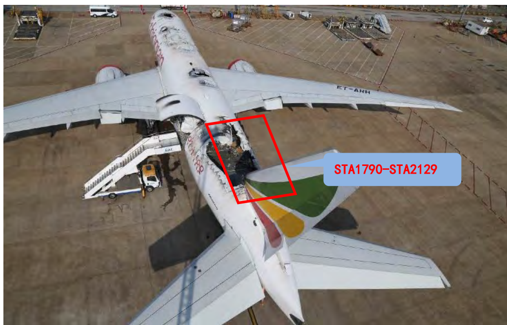
Figure 60 the Largest Burn-through Area of Aircraft Skin
