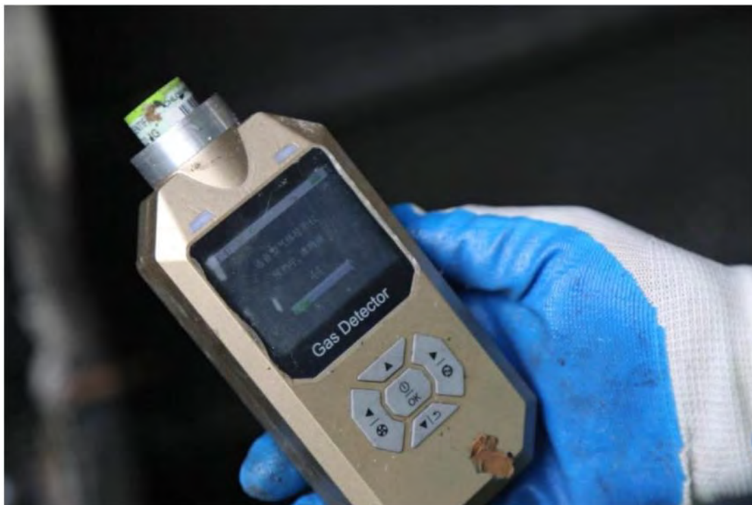
Figure73 Chlorine Dioxide Gas Detector found on Position PR
