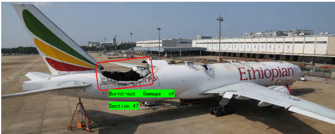
Figure 3 Damage to Upper Fuselage
