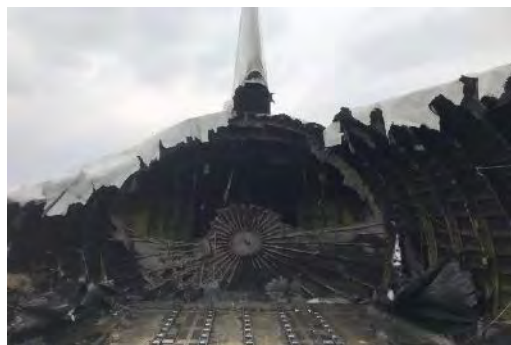
Figure 6 AFT Pressure Bulkhead Damage
