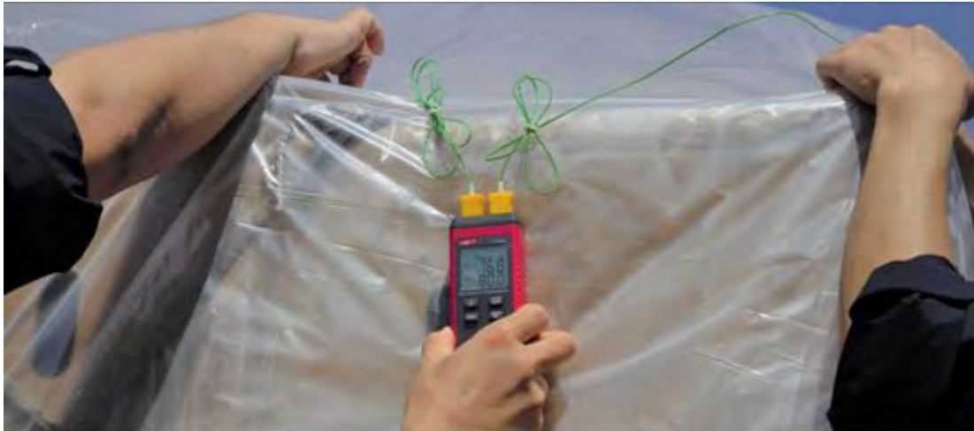
Figure 43 Stack internal temperature
