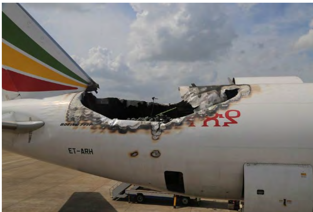
Figure 65 Fire Damage and Heat Discoloration Trace at PR Position (Outer view)
