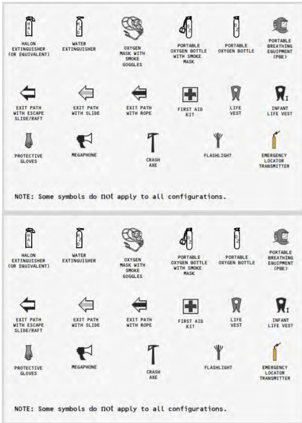
Figure 29 Emergency Equipment Symbols
