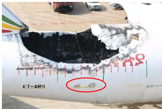
Figure 4 Damage at S24R to S27R
