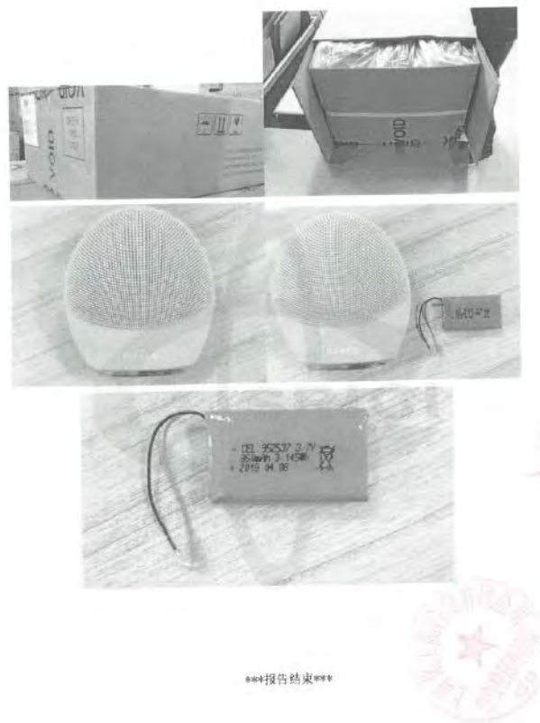
Figure 35 Lithium Battery Carried by the Facial Massager in the Appraisal Certificate
