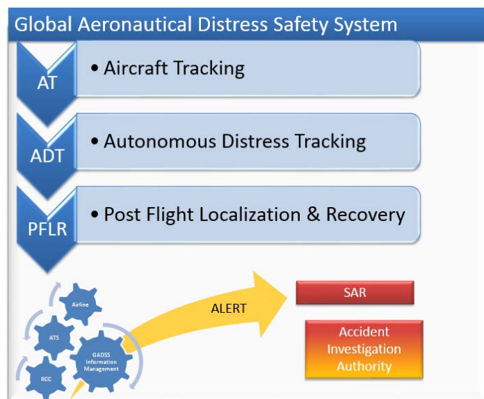
Figure A: high level overview of the GADSS identifying the main functions
